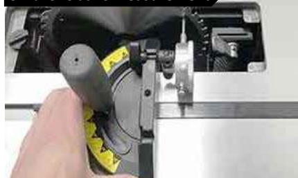
A dedicated saw dial indicator. Such as this one by 'Igaging'
