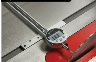
A dedicated saw dial indicator. Such as this one by 'Igaging'
